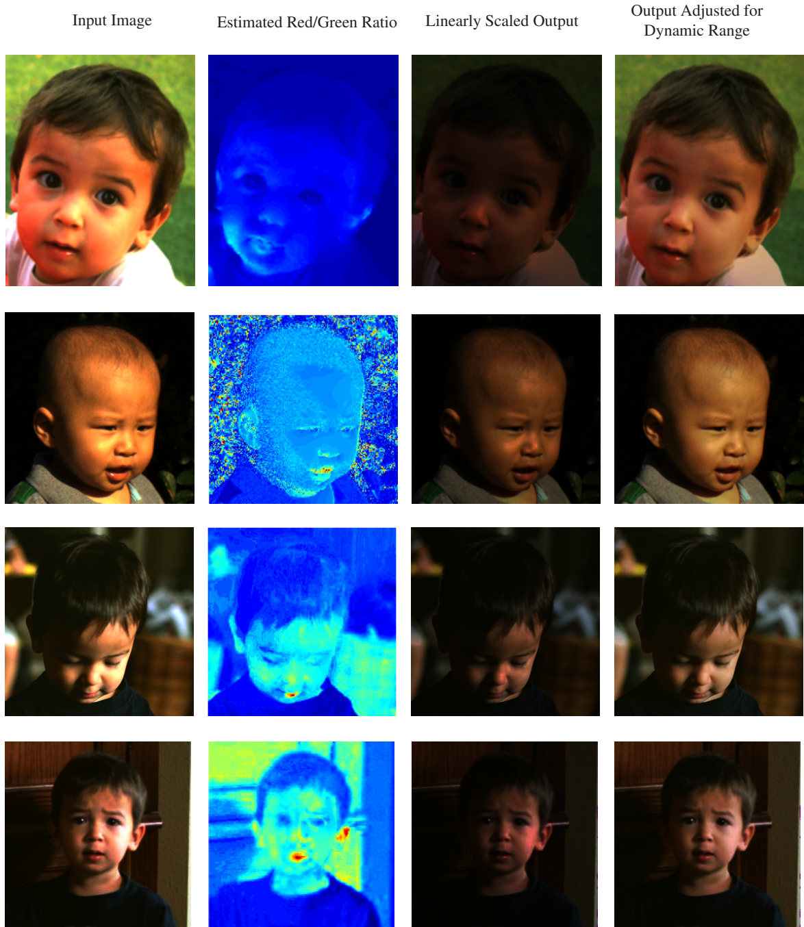
Figure 9: 1st column: Original saturated image. 2nd column: Recovered red:green ratio using the original saturated image. 3rd column: Saturation-free image generated using our method. 4th column: Final result after pixel-wise nonlinear adjustment to the saturation-free image.
